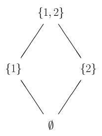
Depicting partial orders ( $\Rightarrow$  p.116) by a such a graph is quite common. Here, node a is below node b and connected by an arc if and only if  $a < (\Rightarrow \text{p.119})b$  and there exists no c with a < c < b.
