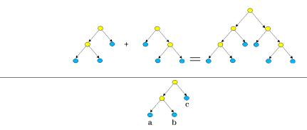
The path  $\langle 0, 0 \rangle$  means: from the root take left subtree, then again left subtree. The path  $\langle 1 \rangle$  means: take right subtree.
