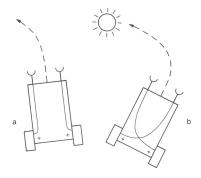
Functionality: sensors **connected directly** to wheels, so that they turn when sensors are activated  $\Rightarrow$  absolutely **reactive**, no processing/reasoning possible!
