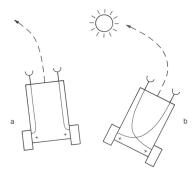
Functionality: sensors connected directly to wheels, so that they turn when sensors are activated ⇒ absolutely reactive, no processing/reasoning possible!
