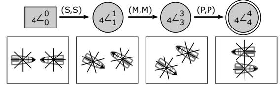
Figure 3: Idealized thread of a rule applied for avoiding head-on collisions between vessels of the same type (acc. ColRegs)
