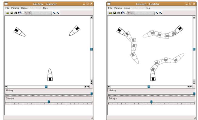
Figure 5: Configurations in the SailAway simulator window; left: an initial situation with three motor vessels; right: the resulting trajectories determined by the system
