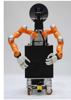
Figure 1: The DESIRE technology demonstrator with two LBR arms (7 DOF) including the four finger anthropomorphic hands (SAH).
