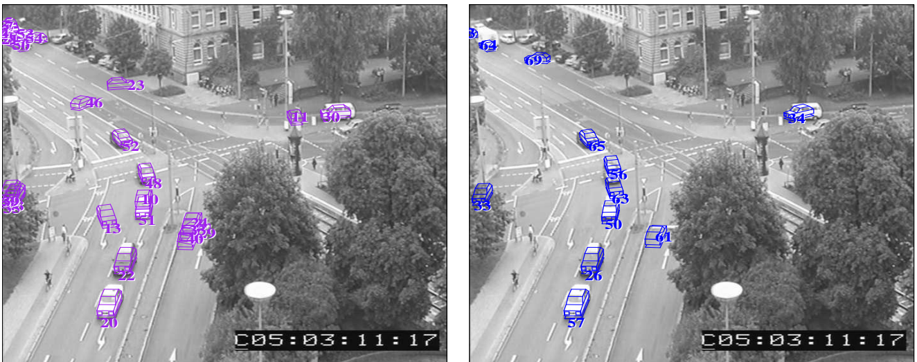
Figure 6. Tracking results at the final frame of the image sequence stau02 . Left: experiment V0. Right: experiment V1. Using qualitative feedback in V1 removes many object candidates which remain in the scene after tracking failed in experiment V0.
