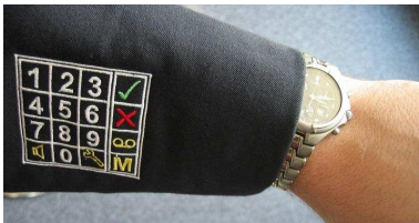
Figure 2: A textile keyboard for aircraft cabin operation.
