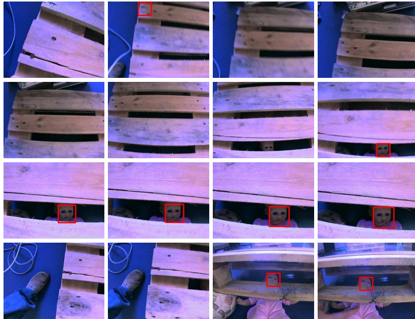
Fig. 6. Series of pictures that demonstrates victim face detection based on ADABOost with simple features.
