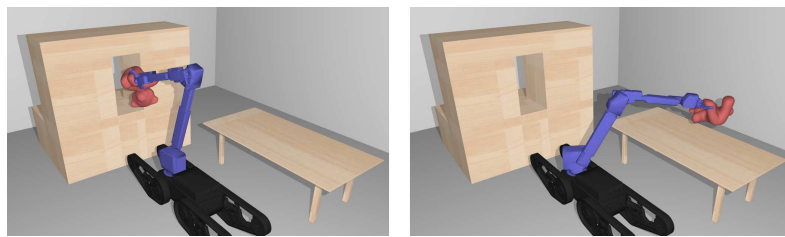
Fig. 4. A pick-and-place task applied to a deformable movable object. The teddy is picked up from behind the wall and moved through the small narrow passage (left) to its final position above the table (right). An execution path can only be found, if deformability of the teddy is considered by the geometric planner.
