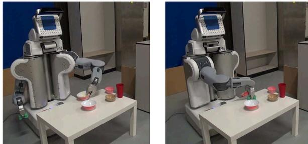
Fig. 1. This figure shows the PR2 robot during the execution of a tidy up task. The robot picks up a bowl to wipe the spot where it was placed.
