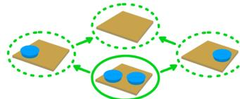
Fig. 2. This figure shows the subsumption hierarchy for successful requests to put an additional object on the table. When a putdown request succeeded on the table with two objects already placed, we can infer that less constrained cases must also succeed without the need to do any calculations.
