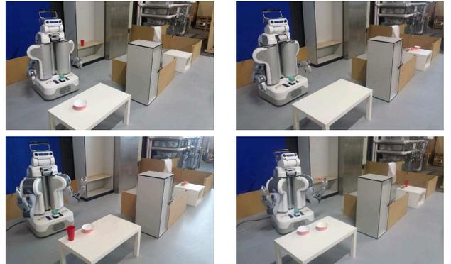
Fig. 3. This figure shows four of the evaluation settings. The task was to bring all objects to the front table and wipe the spot under each object.
