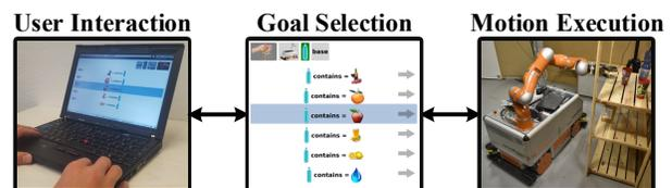
Fig. 1: A user (left) interacts with the goal formulation interface (middle) to control a robotic system (right).
