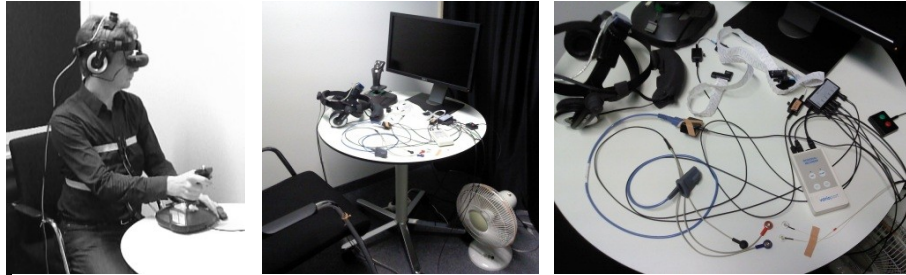
Fig. 2. (left) An example of the complete setup; (middle) The experiment room with HMD, joystick, physiological sensors, fan, and desktop monitor; (right) The "VarioPort" biometrical device with sensors for skin conductance, ECG, finger pulse, and chest measurement, plus remote marker buttons
