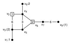
A number on an edge means that there are as many nodes on a line.
