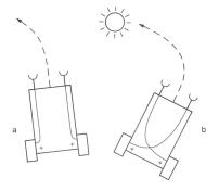
Functionality: sensors connected directly to wheels, so that they turn when sensors are activated  $\Rightarrow$  absolutely reactive, no processing/reasoning possible!
