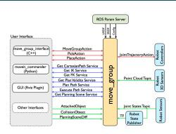
"[The] high-level system architecture for the primary node provided by Movelt! called move\_group, pulling all the individual components together to provide a set of ROS actions and services for users to use."
