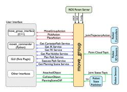
"[The] high-level system architecture for the primary node provided by Movelt! called move group, pulling all the individual components together to provide a set of ROS actions and services for users to use." (http://moveit.ros.org/documentation/concepts/)
