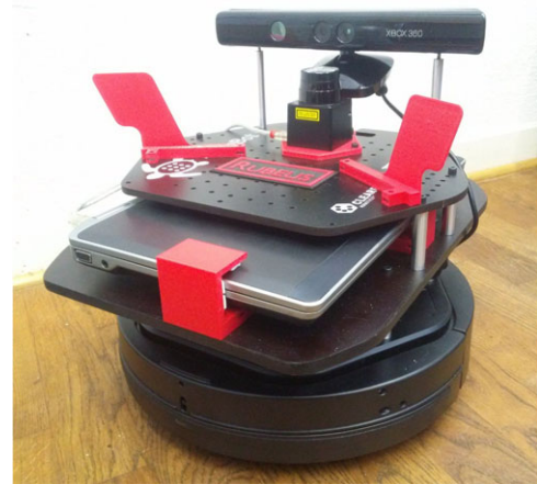
Figure 9. One of the Turtlebot 2 robots used in the experiments with a Kinect sensor and a Hokuyo laser.
