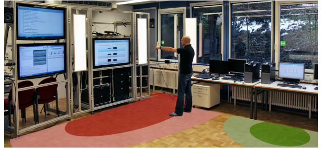
Figure 5: The figure shows the environment in which our prototype system was set up. There is a user making a pointing gesture towards the main terminal of the system. On the left and right side of this terminal, there are laser range finders for user localization (Only the one on the right is part of the picture). On the right is another desktop computer that can be used for user interaction as well. The colored areas depict the discrete locations of the MLN model that is used for user localization.
